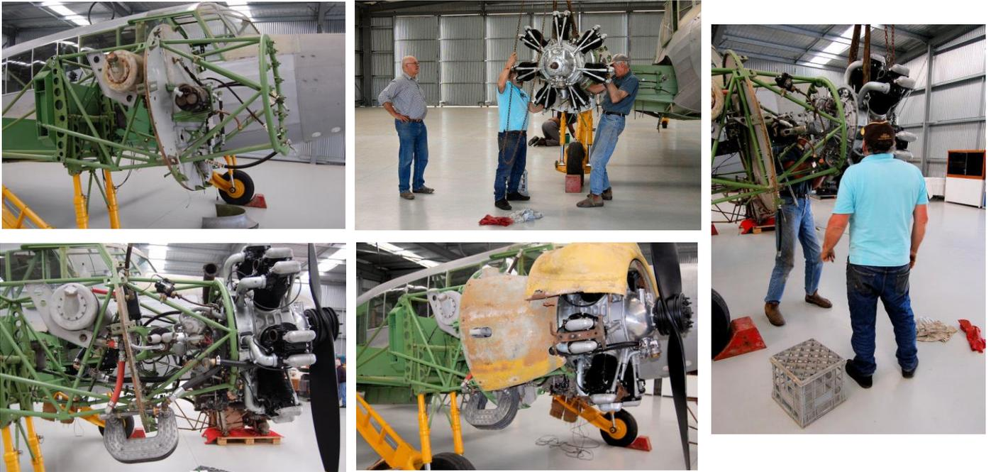
These photos taken during a three month period show the various phases of engine assembly. Attaching the motor took a couple of hours but the finishing touches take weeks.
