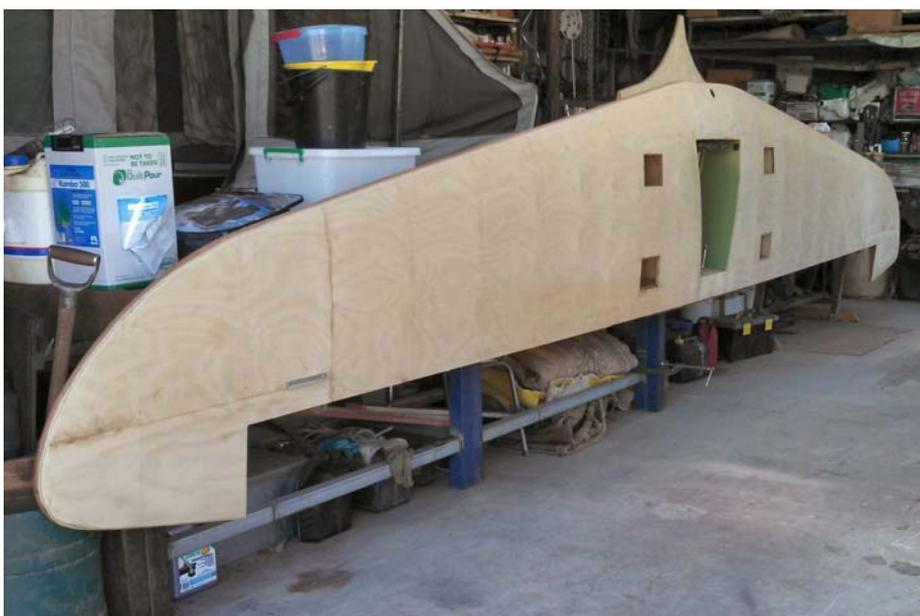
Len Creek has been busy preparing the rear stabiliser for covering with fabric. Some attention to the leading edge and a light sanding should have it ready for covering. However, due to the continual rain and moist weather Len has decided to leave any further work until he is sure the timber is completely dry. This may take another month or so as it is still raining every few days. Elevators fill the gap at the bottom but these may not be fitted until this assembly is fitted to the airframe.
