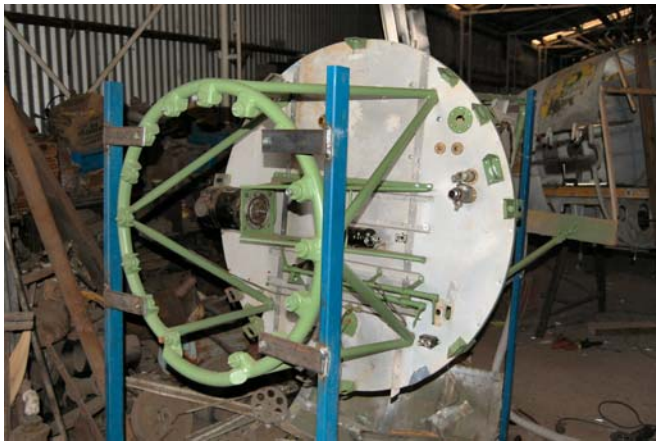
5 & 6. The firewall is ready for dozens of hoses to be attached
