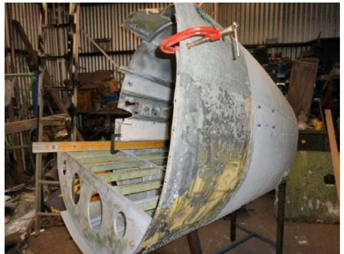
3 & 4. Mick Kingwill is rebuilding the original nose cone that was cut from the cabin with an axe.
