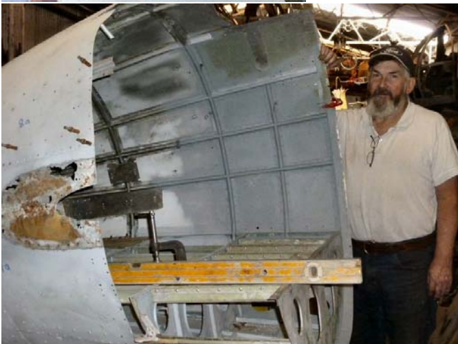
3 & 4. Mick Kingwill is rebuilding the original nose cone that was cut from the cabin with an axe.
