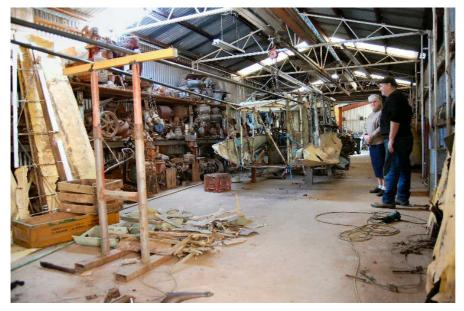
A whole new rear section of fuselage needs to be built. The original steel from this section has been used for farm machinery repairs. Note the two black lengths of tubular steel running to the top left hand edge. This is the start of the new fuselage.
