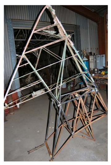
The tail section had been cut in two with an axe many years ago (we are not sure why this was done – perhaps to make it fit on a trailer). Accurate realignment and reconstruction took many hours. The new steel connecting both sections is black. The rudder connects to the right hand side edge of this structure.
